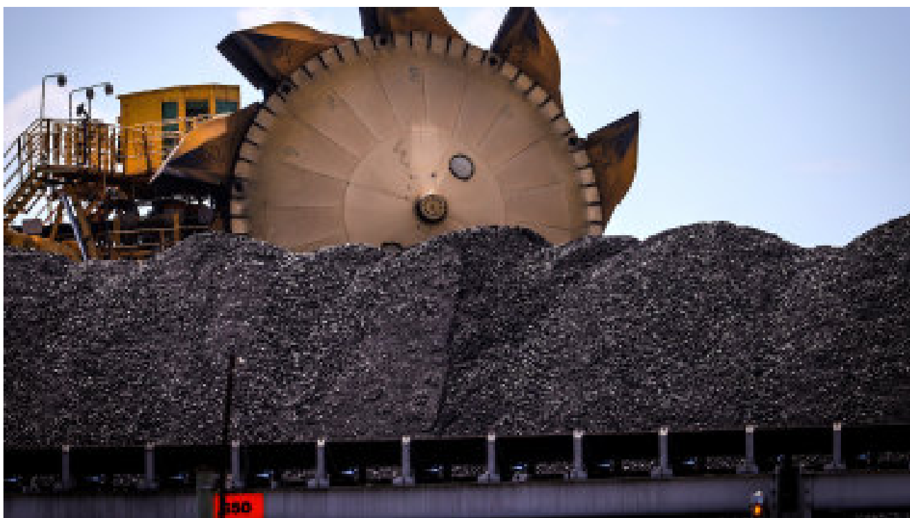
A bucket-wheel reclaimer stands next to a pile of coal at the Port of Newcastle in Newcastle, New South Wales. CREDIT: BLOOMBERG
